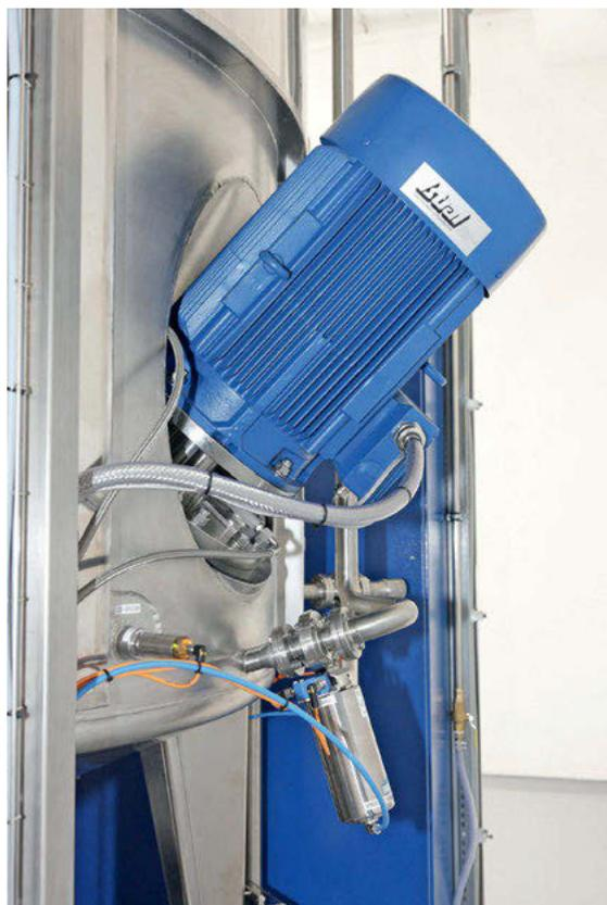
Figure 5: The integrated jet stream mixer
